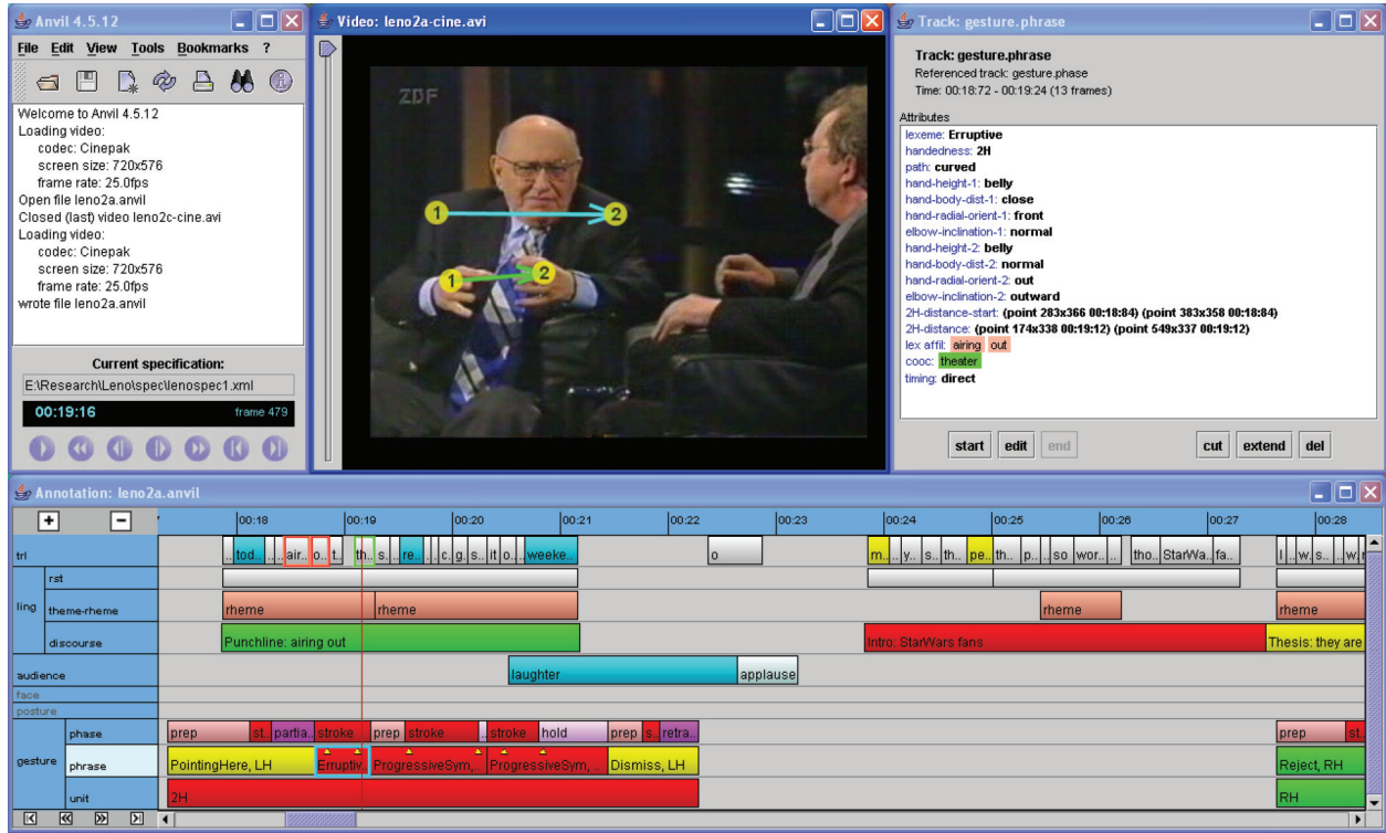
Fig. 5. The ANVIL video annotation tool allows human coders to efficiently encode time-aligned information for digital video. During analysis, a video corpus for each speaker is transcribed for statistical modeling of gesture behaviour. The bottom window contains the multi-track annotation board where coding takes place.
